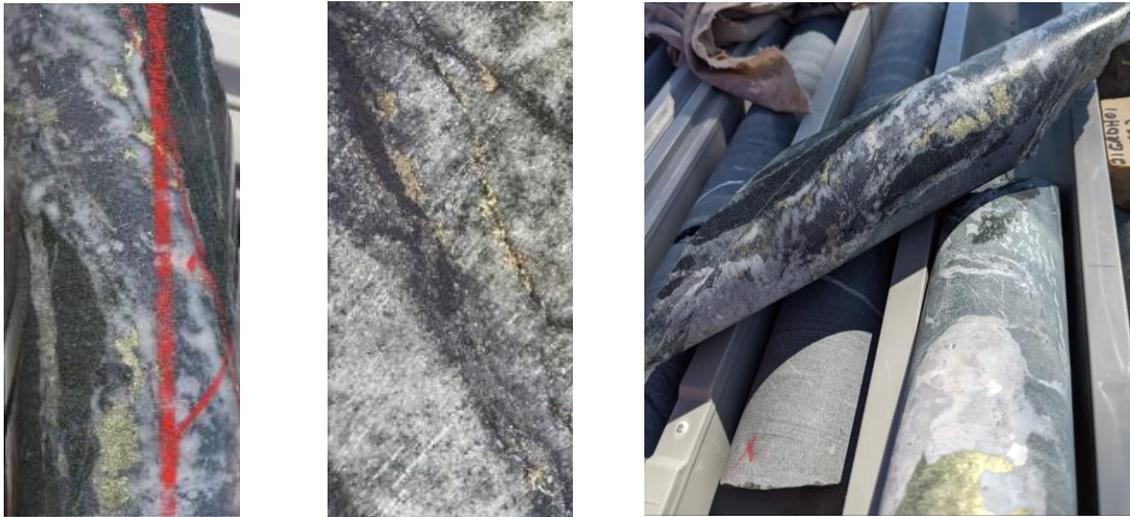
**Figure 1:** Osprey IOCG copper mineralisation (chalcopyrite) in drill core.<sup>3</sup>
