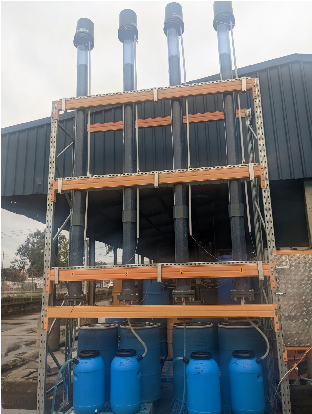
Figure 7 - Column Leach Testing at Brisbane Met Labs
