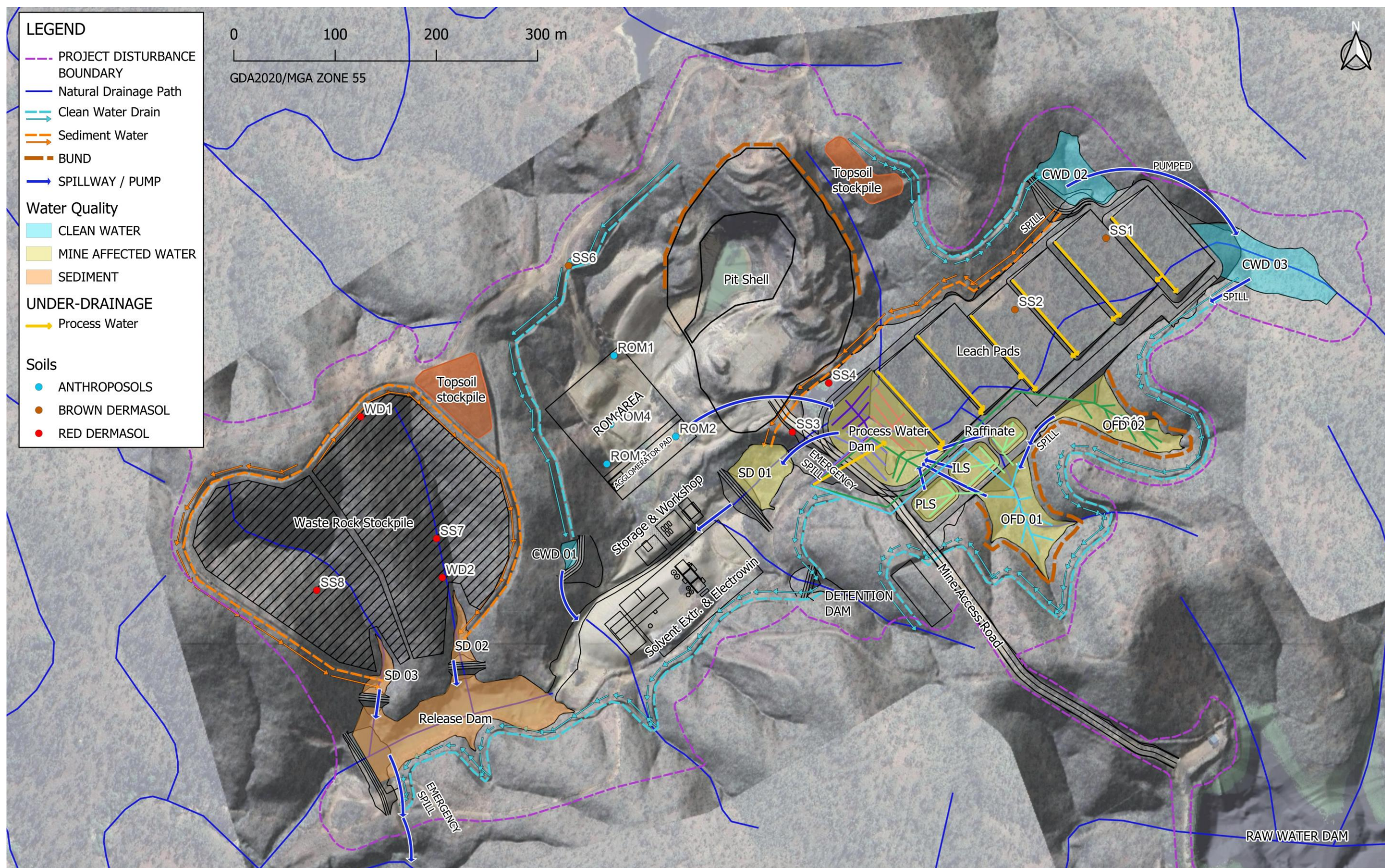
Figure 6-2: Layout showing Spill/Pump Direction
