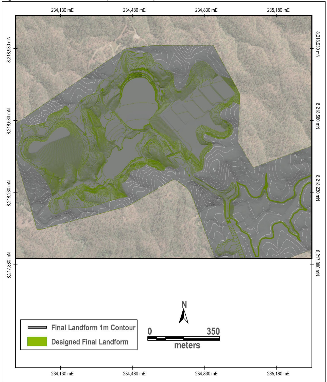
Figure 10: Final Landform 3D (section 2.4.5)
