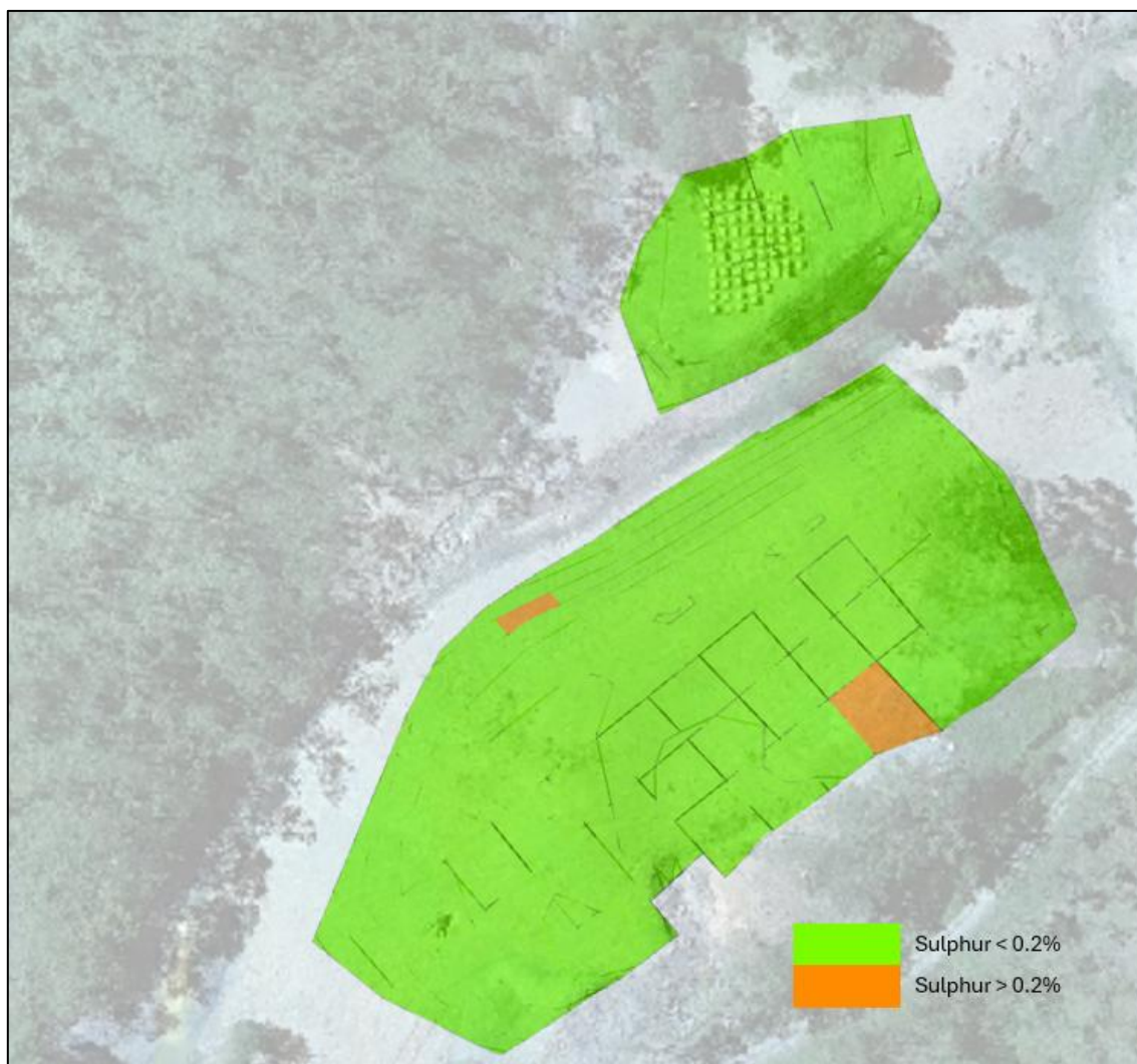
Figure 2 - Existing Waste Rock Stockpile Block Model Split by Sulphur Content
