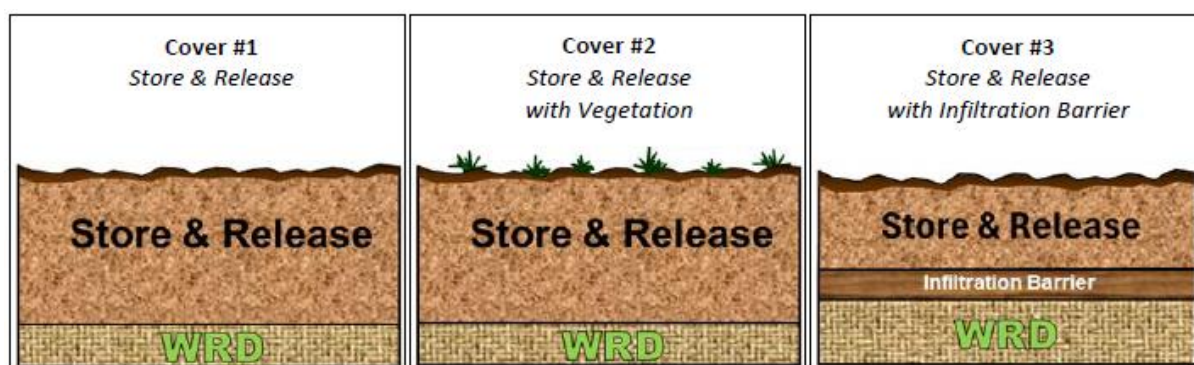
Figure 11: Closure conceptual layering for modelled store and release cover variations
